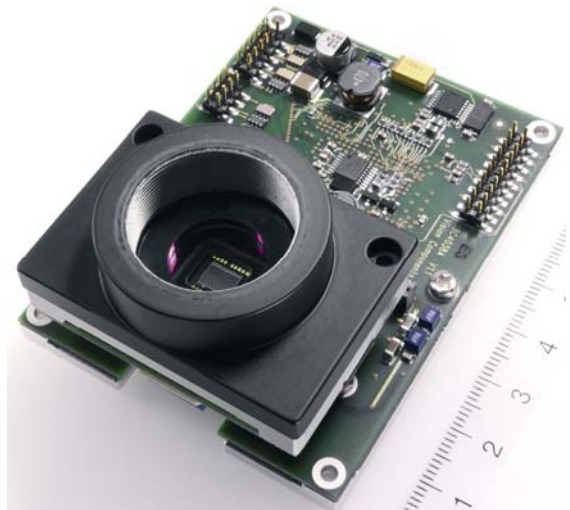
VCSCB40XX Single Board Camera with mounted sensor board (standard delivery) 1
