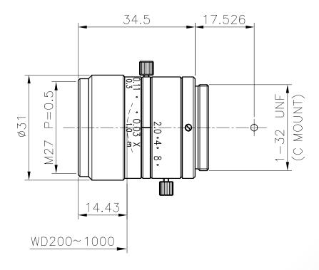
The C-Mount lens Lensagon CMFA3020ND is suitable for common sensors up to 1 megapixel with an image format of 2/3 inch. It is characterized by a particularly high light intensity.
