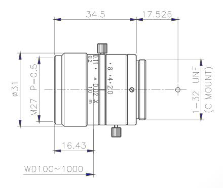
The C-Mount lens Lensagon CMFA2020ND is suitable for common sensors up to 1 megapixel with an image format of 2/3 inch. It is characterized by a particularly high light intensity.
