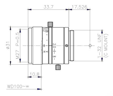
The C-Mount lens Lensagon CMFA1520ND is suitable for common sensors up to 1 megapixel with an image format of 2/3 inch. It is characterized by a particularly high light intensity.
