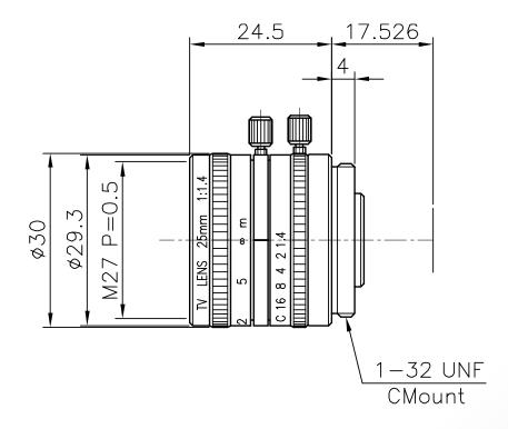
The C-Mount lens Lensagon CY2514 is suitable for sensors below 1 megapixel with an image format of 2/3 inch. It is characterized by a particularly high light intensity.
