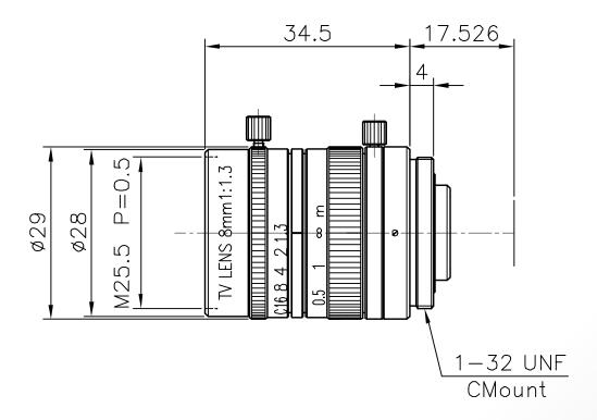
The C-Mount lens Lensagon CY0813 is suitable for sensors below 1 megapixel with an image format of 2/3 inch. It is characterized by a particularly high light intensity.
