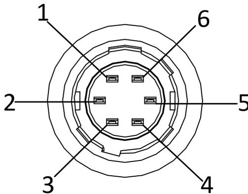
Figure 1-5 Power and I/O Interface
