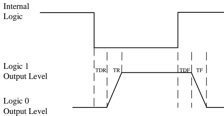
Figure 3-54 Output Logic Level
