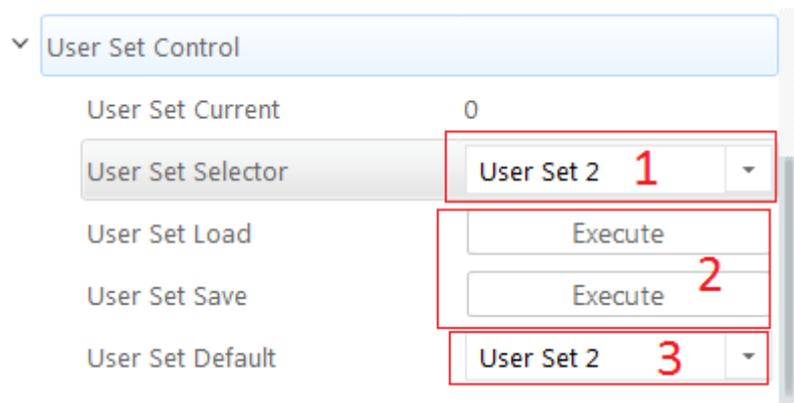
Figure 3-55 Parameters Saving And Loading
