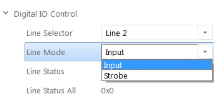
Figure 3-29 Configuring Line 2 Pin to Input
