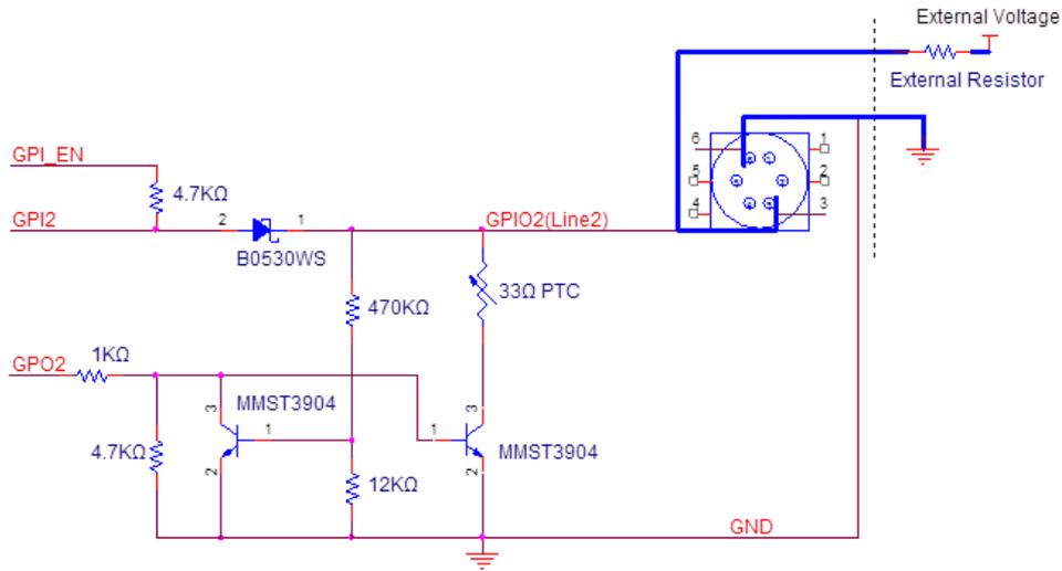
Figure 3-52 Line2 Bi-direction I/O Circuit
