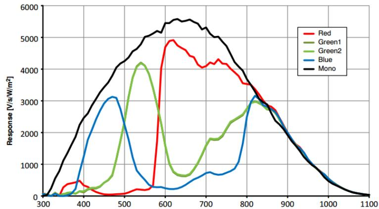
Figure 1-2 MV-CA050-20UM/UC Quantum Efficiency
