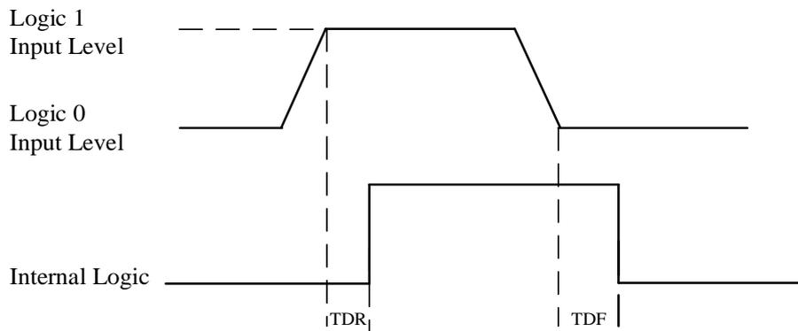
Figure 3-53 Inputting Logic Level
