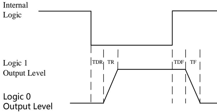
Figure 3-51 Output Logic Level
