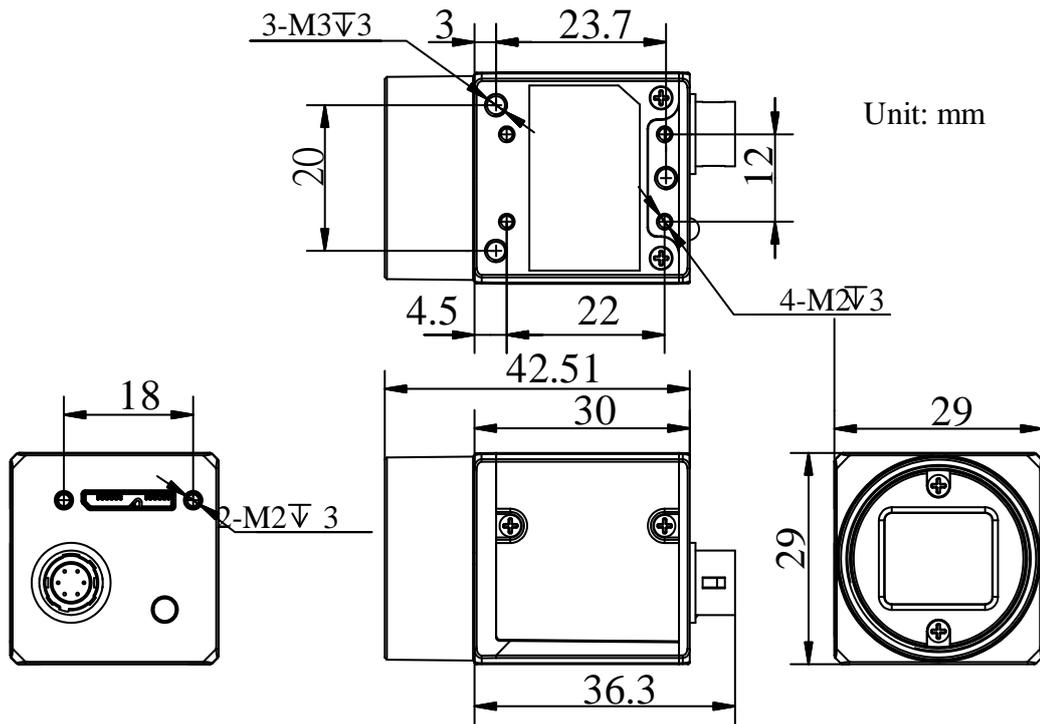
Figure 1-3 Dimension of MV-CA013-20UM/UC and MV-CA050-20UM/UC
