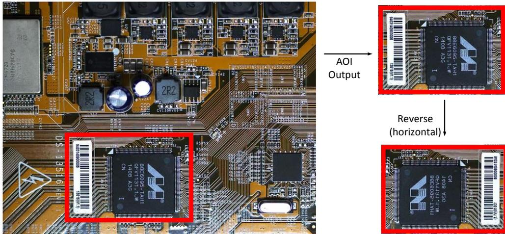
Figure 3-40 The Comparison of ROI Output Before And After Mirroring
