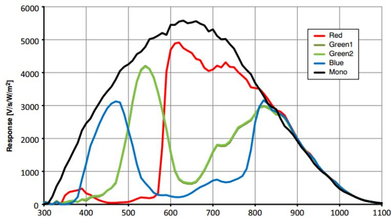
Figure 1-1 MV-CA013-20UM/UC Quantum Efficiency
