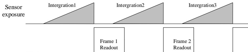
Figure 3-12 Internal Trigger Mode
