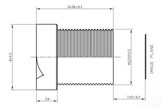
The S-Mount lens Lensagon BT6020V2 is suitable for sensors below 1 megapixel with an image format of 1/3 inch. It is characterized by a particularly high light intensity.
