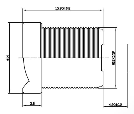
The S-Mount lens Lensagon BT3620C is suitable for sensors below 1 megapixel with an image format of 1/3 inch. It is characterized by a particularly high light intensity.
