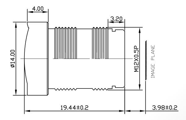
The S-Mount lens Lensagon BT2520C is suitable for sensors below 1 megapixel with an image format of 1/3 inch. It is characterized by a particularly high light intensity.
