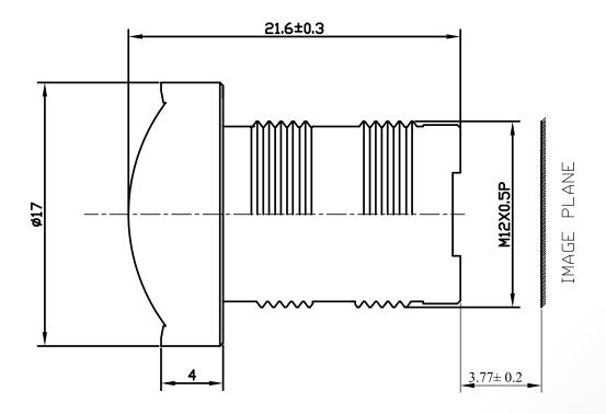
The S-Mount lens Lensagon BT2120C is suitable for common sensors up to 1 megapixel with an image format of 1/3 inch. It is characterized by a particularly high light intensity.
