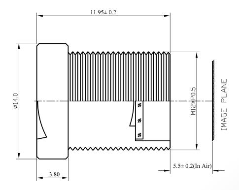
The S-Mount lens Lensagon BT16020NC is suitable for sensors below 1 megapixel with an image format of 1/3 inch. It is characterized by a particularly high light intensity.
