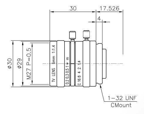
The C-Mount lens Lensagon CY0614 is suitable for sensors below 1 megapixel with an image format of 1/2 inch. It is characterized by a particularly high light intensity.
