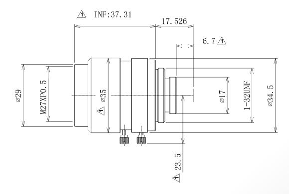
The C-Mount lens Lensagon C3M1216V2 is suitable for common sensors up to 3 megapixel with an image format of 2/3 inch. It is characterized by a particularly high light intensity.
