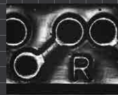
Coaxial spot lighting
